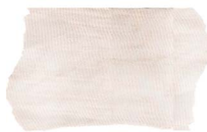
Plate (9) showing cloth piece stained with chocolate and treated with Ariel detergent only at 40°C.
