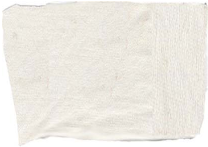
Plate (8) showing cloth piece stained with chocolate and treated with Ariel detergent and St. endus Salh-40 protease at 40°C.
