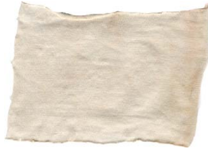
Plate (7) showing cloth piece stained with blood and treated with Ariel detergent only at 40°C.
