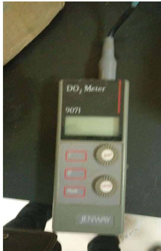
Figure 1-16 Photo of DO meter
